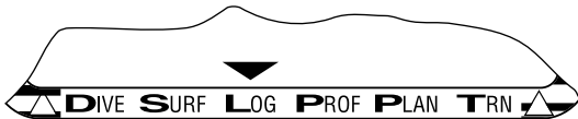
Figure 2: The Mode Indicator makes it easy to determine which mode the IQ-600 is currently displaying.
